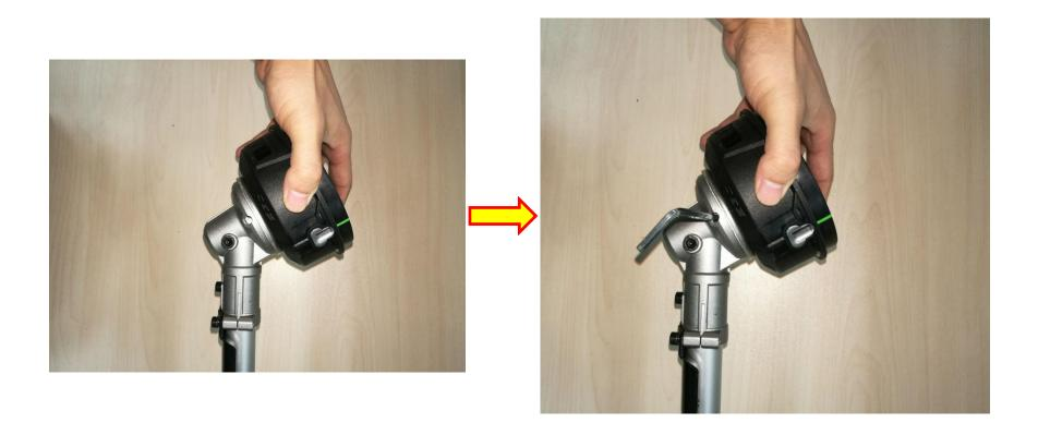
6. Loosen the nut with multifunction wrench clockwise to remove it from the shaft.
