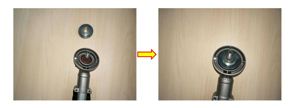
21. Mount the flange cover onto the shaft.
