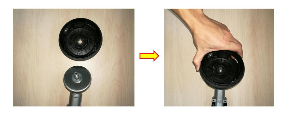
23. Mount the plain washer onto the shaft.
