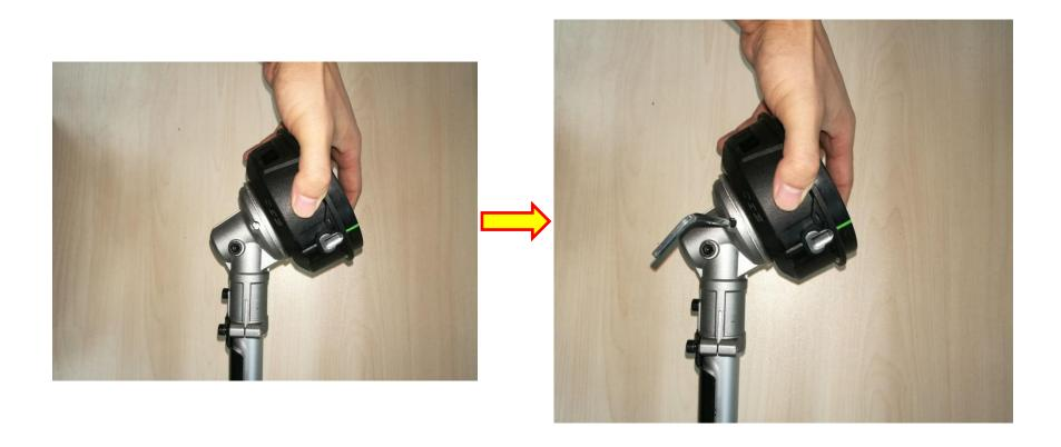
26. Mount the nut onto the shaft and tighten it with multifunction wrench anticlockwise.
