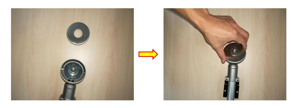
22. Mount the upper housing assembly onto the shaft.
