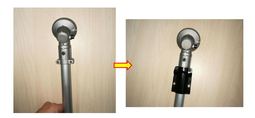
20. Mount the flange onto the shaft.
