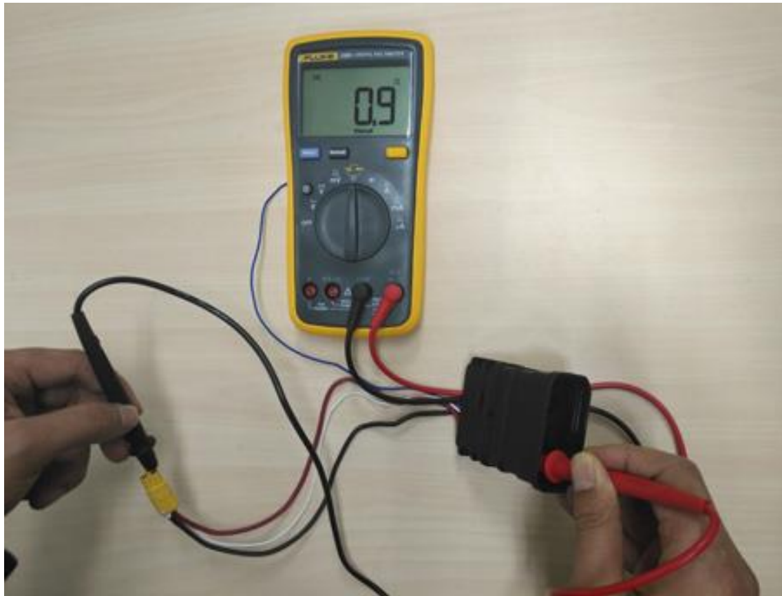
Internal Wire Assembly Measurement
