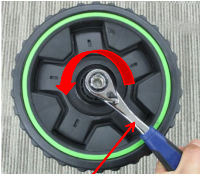
1/2 inch (S=13mm) socket wrench
