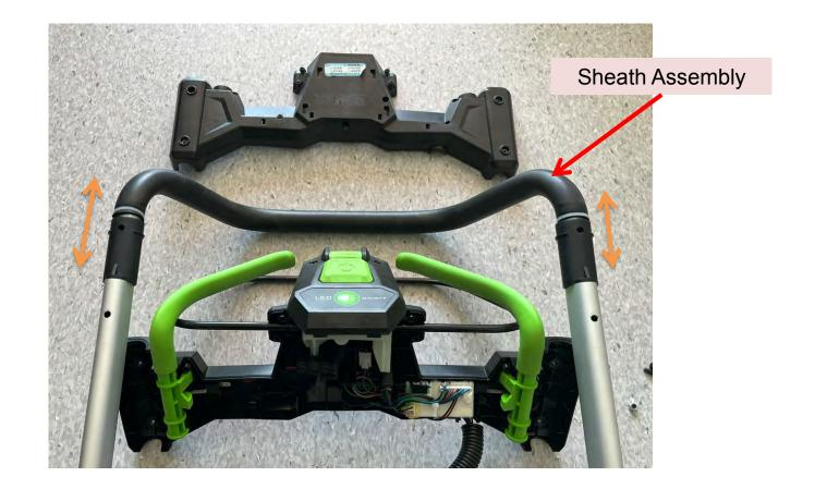
22. Mount the sheath assembly with the tubes into the switch box housing. Making sure that the four locating holes are aligned.
