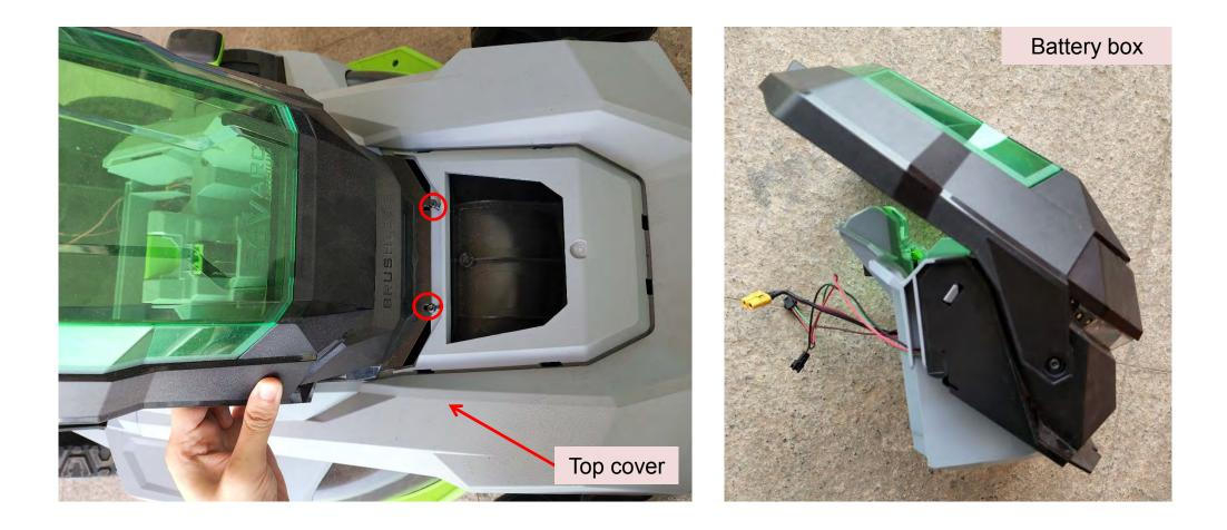
If the battery connector assembly is detected as defective, follow below step 1 ~ 4 to have replacement.
