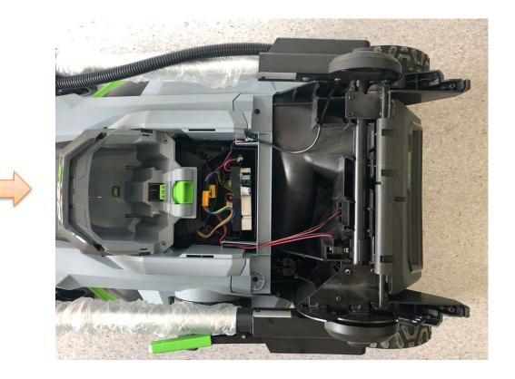
2. Remove the shaft bolt, washer, blade and the fan from the motor shaft as instructed in "Part 1\_Blade Replacement".
