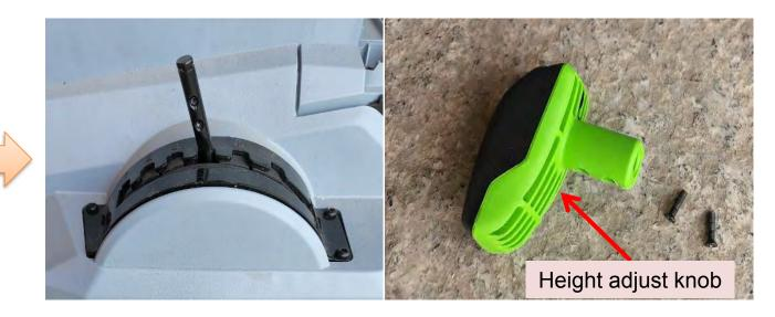
4. Remove the depth stop plate as well as the rubber pad beneath from the top cover by loosen 3 screws.
