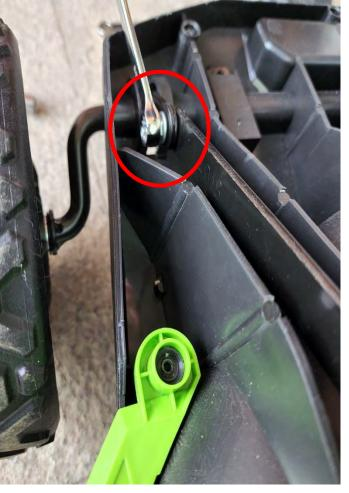
18. Close the top cover and tighten it with the deck using 12 screws.
