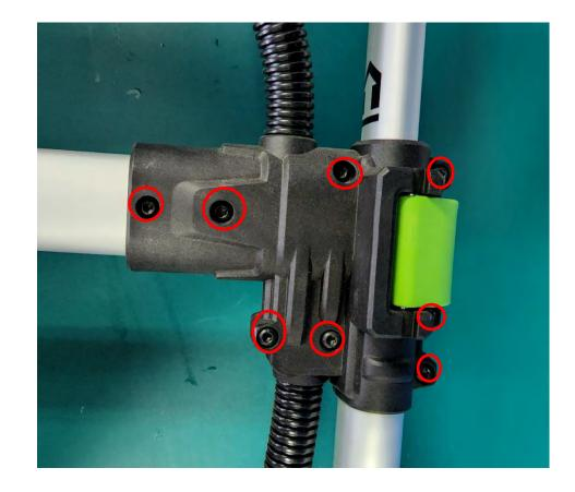
2. Remove the top and bottom cover, rubber block and clamp block. If the rubber block or the clamp block is damaged/worn, replace it with a new one directly. If the covers are damaged, replace the whole right cover assembly (marked red) with a new set.
