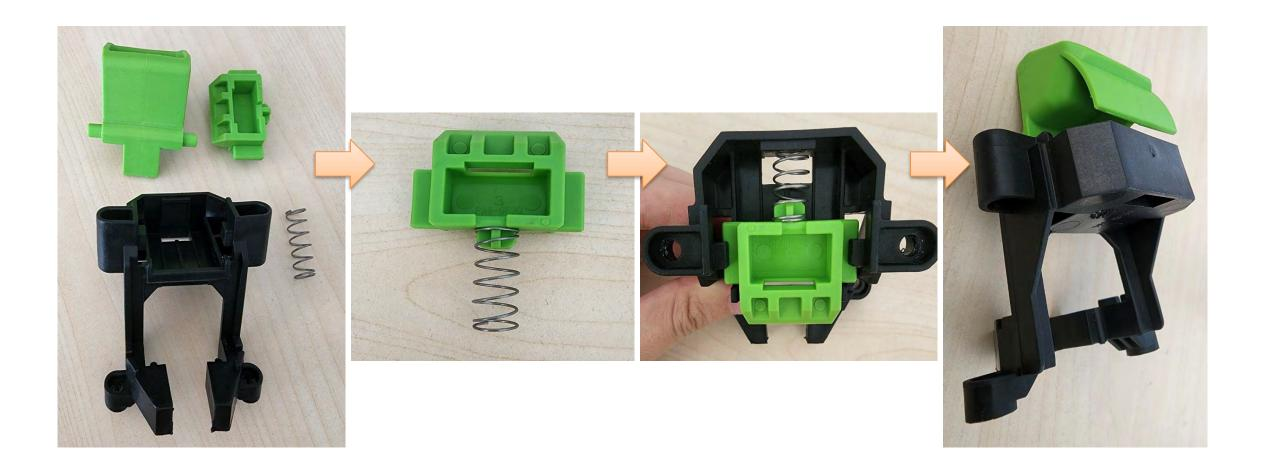
③ Mount the new seat wire assembly into the battery latch assembly.
